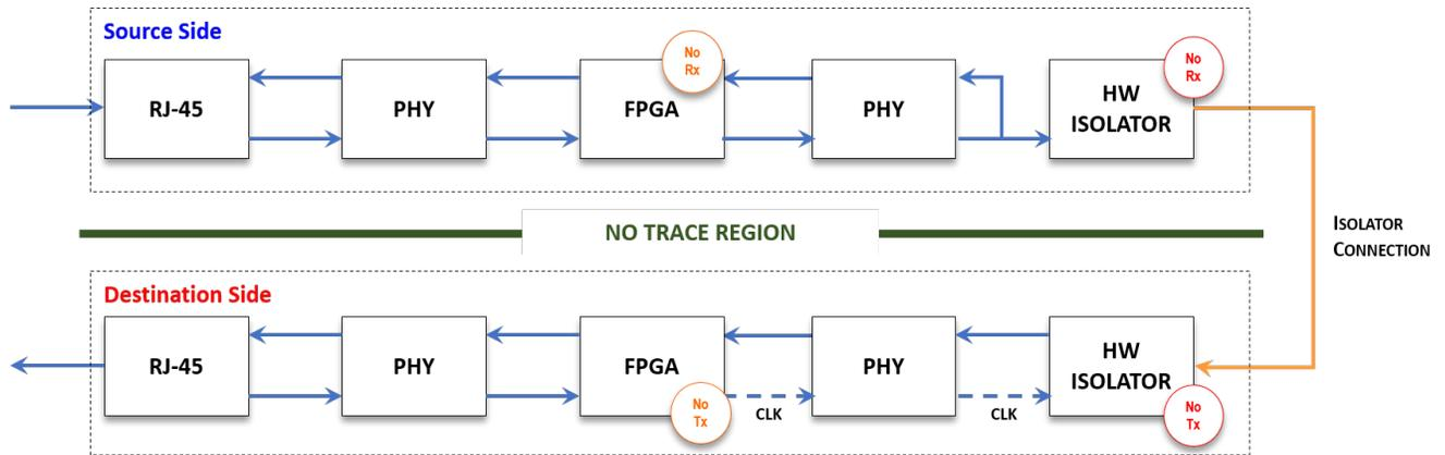
**Figure 8 – Architectural Block Diagram Showing Inter-Component Communication and One-Way Flow Control from Source to Destination**
