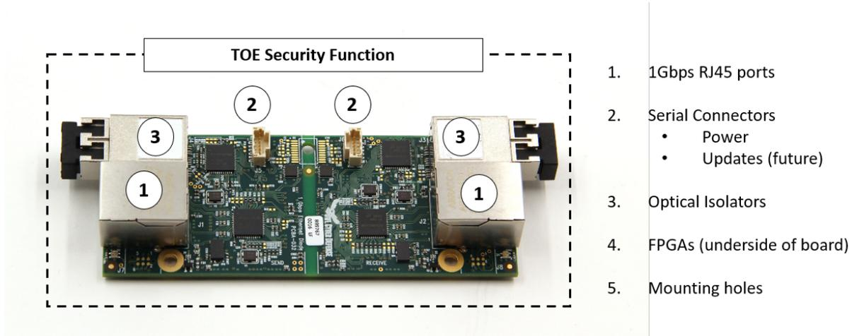
**Figure 5 - XDE Radium Optical Model Top-Down View with Major Components Identified**
