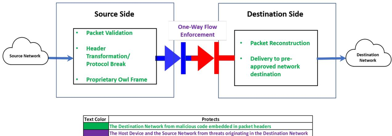
Figure 1 - XDE Radium Protection Features
