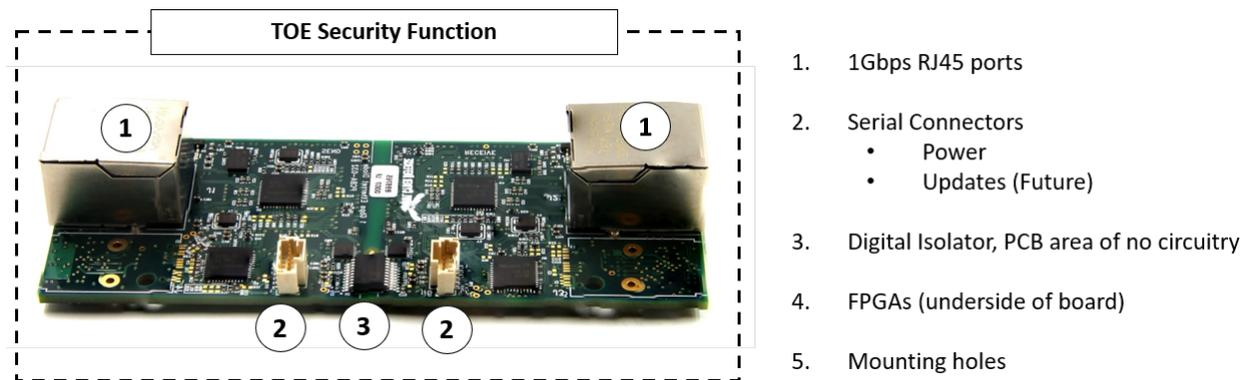
**Figure 6 – XDE Radium Digital Model Top-Down View with Major Components Identified**
