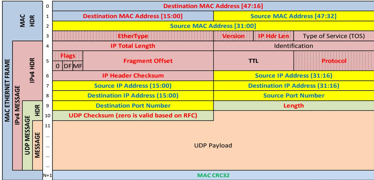
**Figure 3 – Standard Ethernet Frame Received by XDE Radium**
