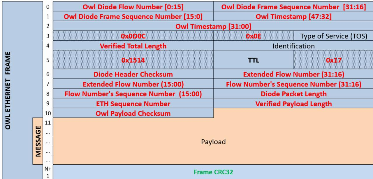
**Figure 4 – Owl Proprietary Frame delivered to the Hardware Isolator**
