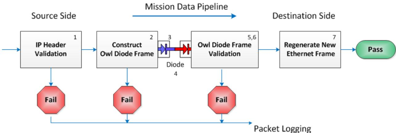
**Figure 2 – XDE Radium Ethernet Frame Evaluation and One-Way Flow Enforcement Scheme**
