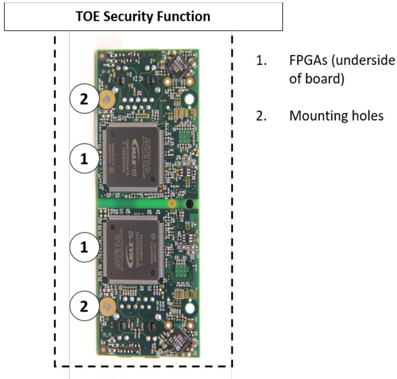
**Figure 7 - XDE Radium Bottom View with Major Components Identified (Components and Lay-Out Common Between Optical & Digital Models)**
